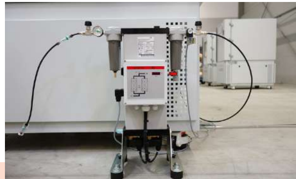
Compressed Air Dryer
