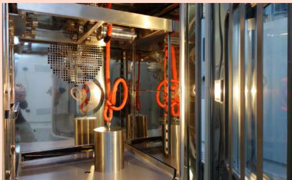
Cold Bend Cables Testing
