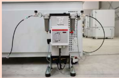
Compressed Air Dryer
